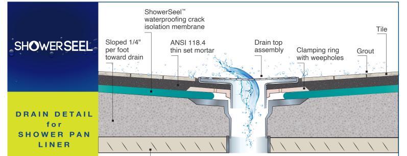
Substrate concrete, or wood
